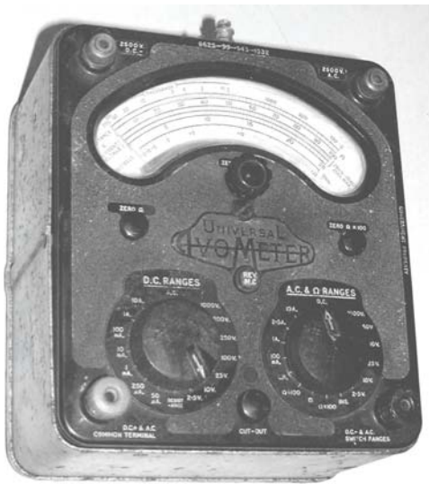
Avo Model 8, Z4/6625-99-943-1532 with metal panclimatic case
