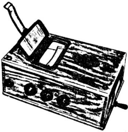
Tester, Insulation, No.1 in its teak box over 14 inches long
