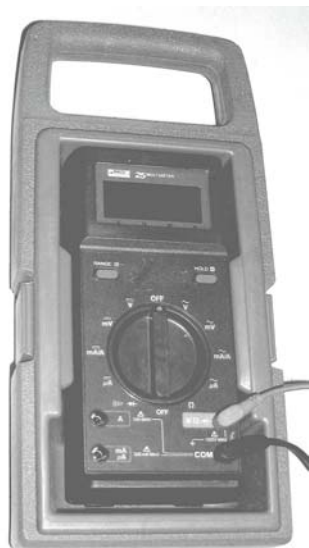
A Fluke digital multimeter Z4/6626-99-252-3606 well protected for military service
