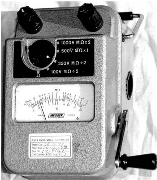
Megohmmeter Type 70154 Mk 2, (Z4/6625-99-325-2217). Note that with increasing voltage, higher resistances can be measured.
