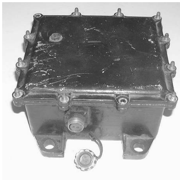
Generator Panel No.9 Mk 4 looking much like earlier panels except the additional two-pin socket.
