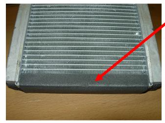
Attach seal to last 2 rows of Heater Core
